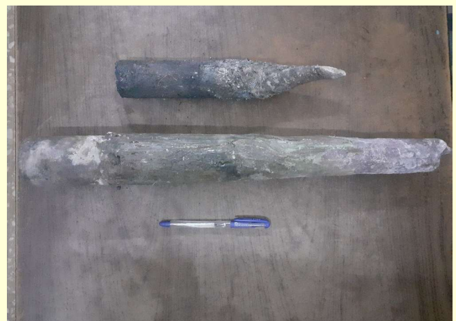
Figure 2: Corroded molybdenum electrode
