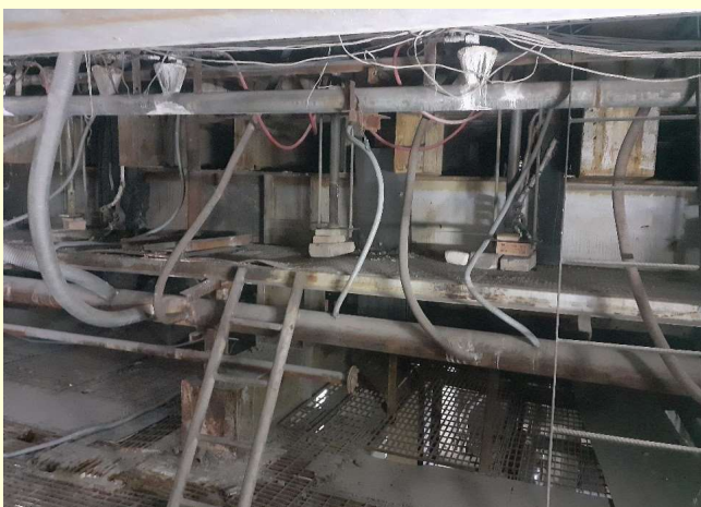
Figure 1: Electrodes positioning in glass melting
