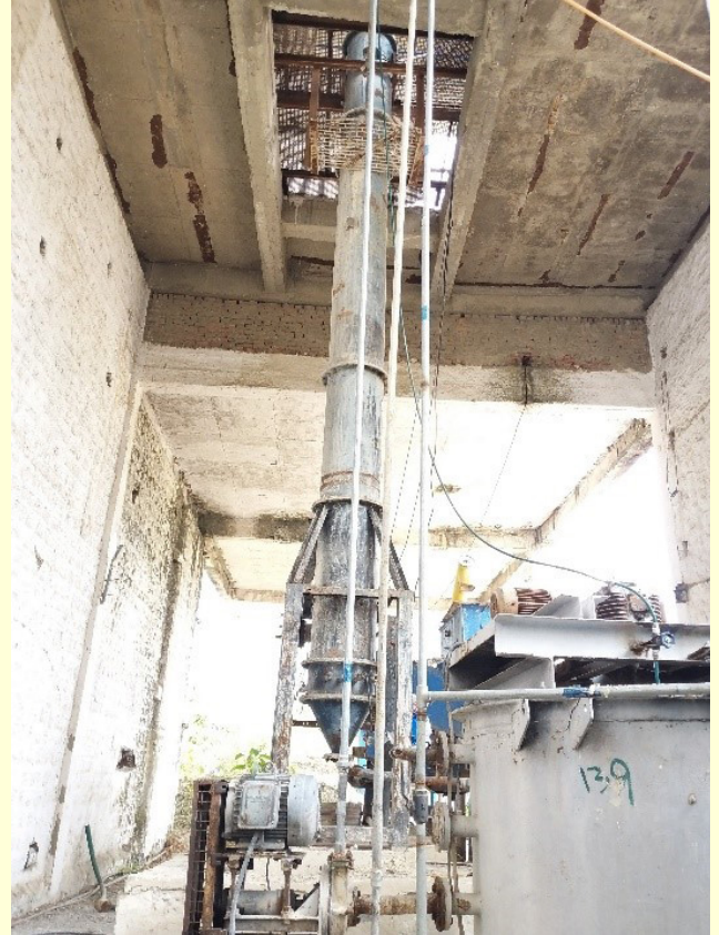
Figure 1: 25 tonnes per day capacity NML flotation column (0.5m diameter) installed at M/s Vedam Calcimin Pvt. Ltd., Telangana for beneficiation of limestone.
