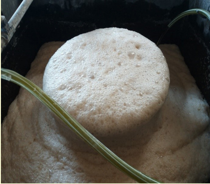
Figure 2: Collection of froth/concentrate of limestone using eco-friendly flotation reagent
