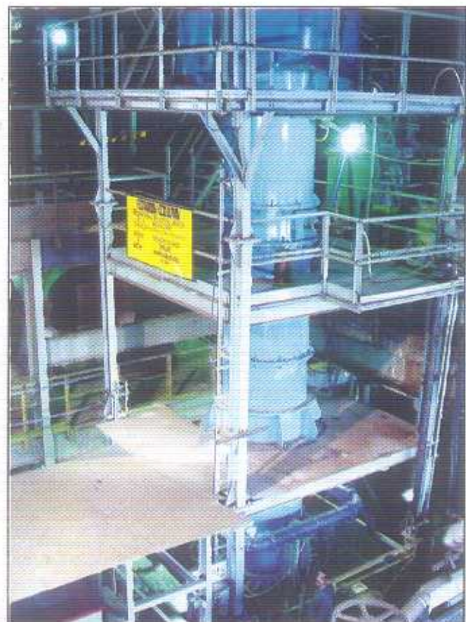
NML's flotation column under operation at Indian Rare Earths Ltd., OSCOM, Chattrapur.
