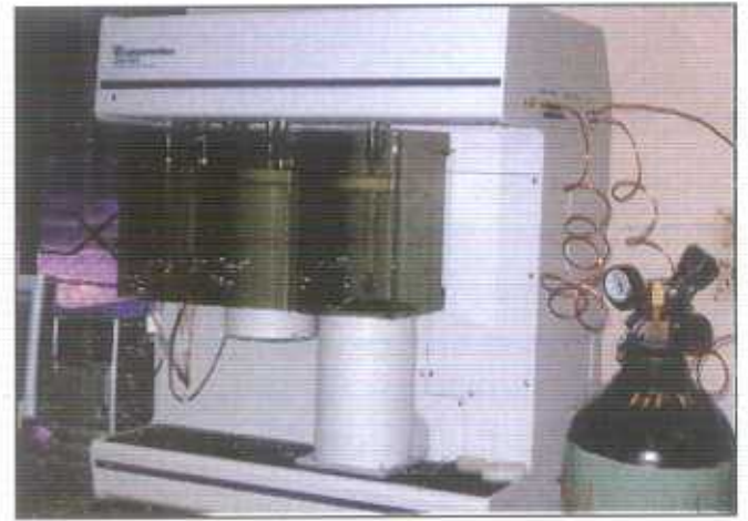
BET Surface Area Analyser (Micrometrics, USA) installed at NML Madras Centre
