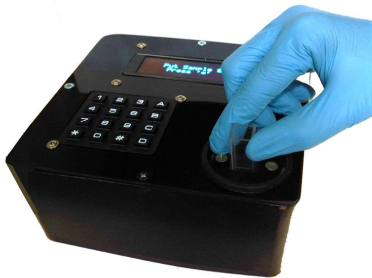
Fig: A schematic of prototype of Fluorescence based HCHO tester
