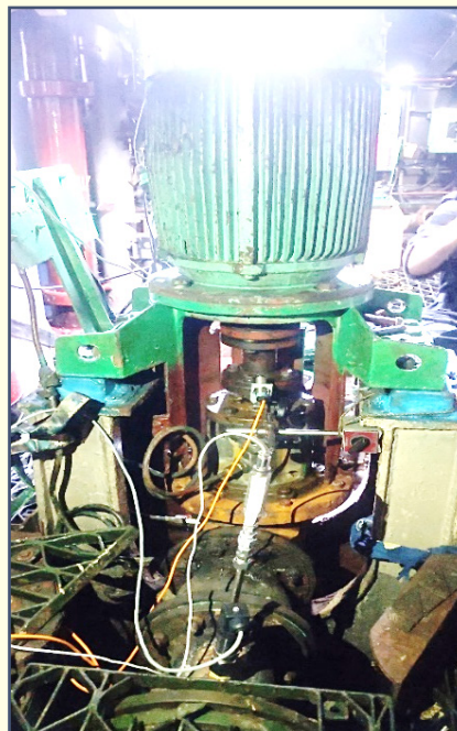
Pressure Probes installed at Suction and Discharge Side of the pump Assembly Speed sensor mounted with a magnetic stand Power Tapping from the Pump-Motor Discharge Side of the pump Assembly
