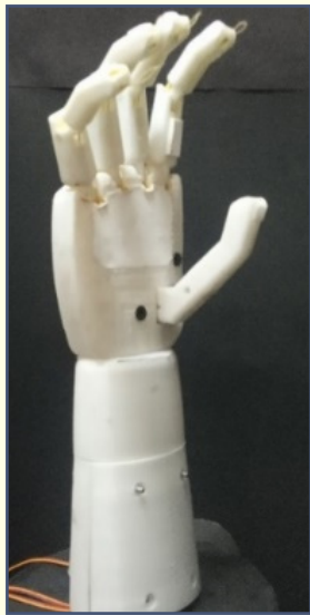
Fig 1. Prosthetic hand prototype Fig 2. Demonstration of grasp classification by prosthetic hand (a) Pinch grasp (b) Tripod grasp (c) Power grasp
