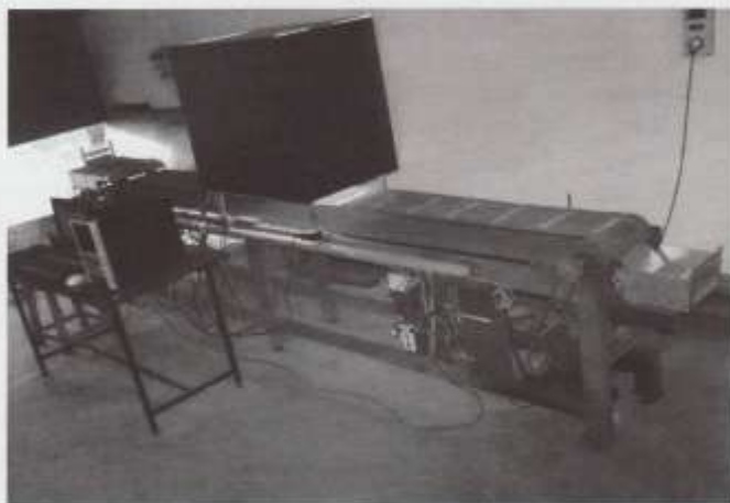
Figure 6. Smart-camera based machine vision system for real-time inspection and sorting of biscuits
